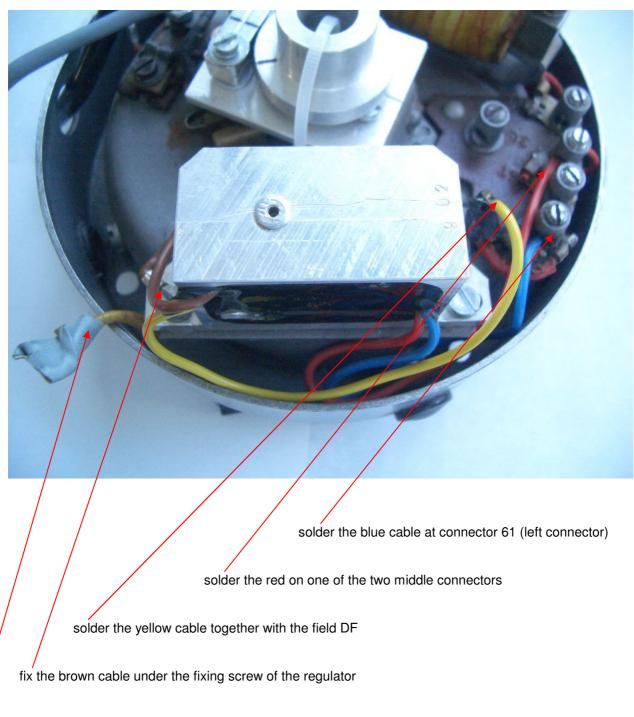
this is the connector of the resistor, leave this disconnected and isolate it
